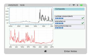
SmartID uses SSP to provide a singular, confidencebased result. Check marks indicate the result was confirmed by both Raman and FTIR.
