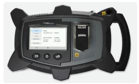
The VipIR is a lightweight, handheld device that utilizes SSP, FTIR, and Raman technologies to identify thousands of chemicals.
